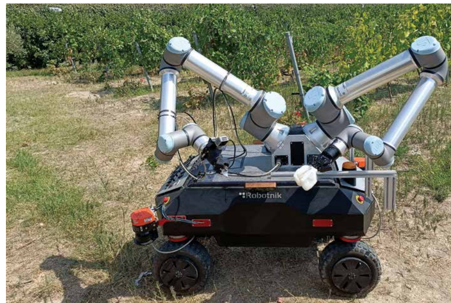
Above: Cropsy AI-powered vine scanner that attaches to a vehicle to detect early signs of diseases such as mildew. Right: A prototype of a grape-harvesting robot seen in Greece uses AI to identify ripe, healthy bunches. Facing page: Cork Supply using AI with a scanner to view the internal structure of corks and identify their OTR (Oxygen Transmission Rate)
